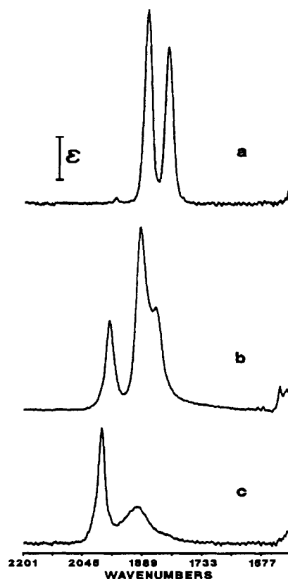
Figure 7. IR spectra of (a) 1.12 mM 3 , (b) 2.27 mM 3^+ , and (c) 1.12 mM 13^{2+} in \text{CH}_2\text{Cl}_2 at 203 K.
